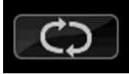
**Press and hold the transfer button for 3 seconds** to affect a transfer. This transfer touch zone can be removed if desired (to make the install more secure) via the "Control" menu and selecting the "Allow Transfer", "OFF" option. The unit can still be transferred using the priority switch at the rear of the STS.
