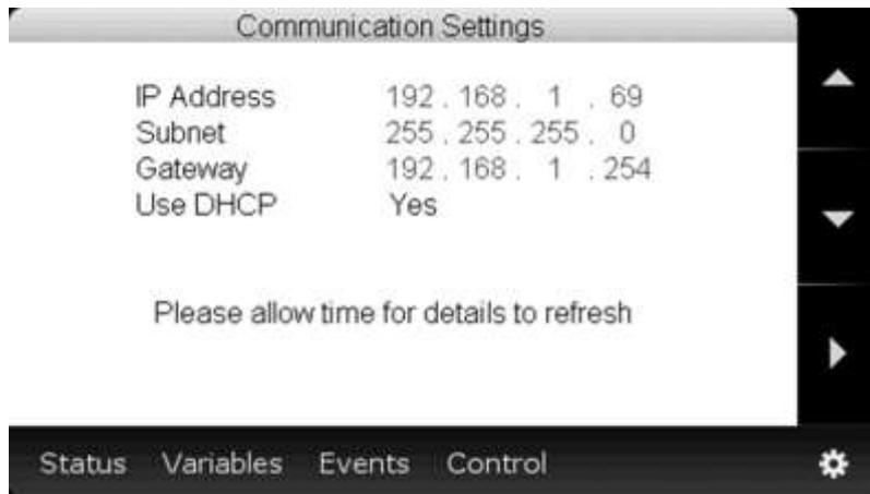
LAN Web Server and SNMP TCP / network address configuration.
