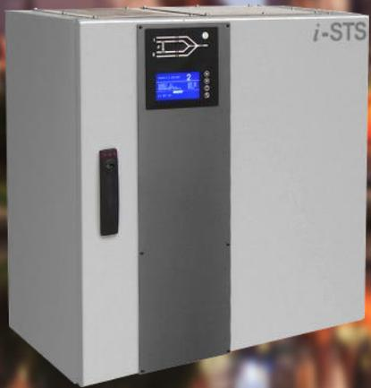
Each unit has a triple redundant power supply module. Only one power supply is required to operate the STS. Power supplies 1, 2, 3 have their own source of AC power which are Input Source 1, Input Source 2 and Output respectively. Each power supply has an extended operating range from 85 to 305VAC and are frequency insensitive.
